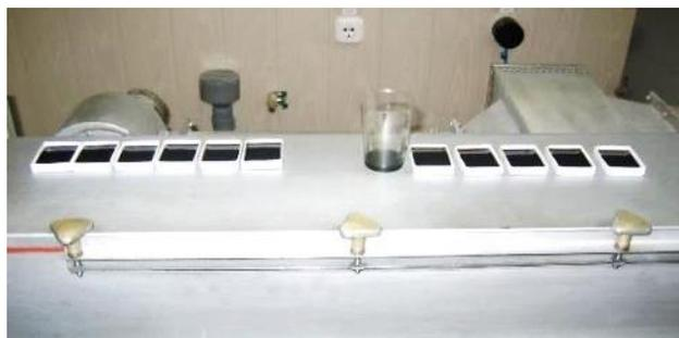
**Figure 3.** Samples of the epoxy basalt-filled oligomer prepared for processing in a microwave EMF.
