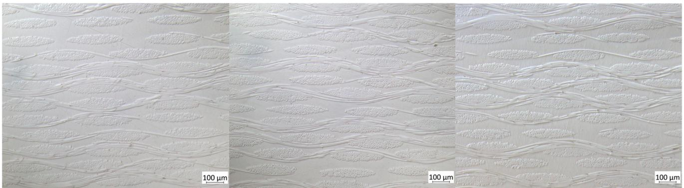
**Figure 9.** Optical microscopy images of tGFRP plate 1 (left), 2 (middle), 3 (right).
