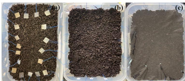
**Figure 1.** Preparation of samples for the biodegradation test in soil: (a) samples arranged on 300 g of soil in a container; (b) samples covered with another 300 g of soil; (c) container covered with foil.
