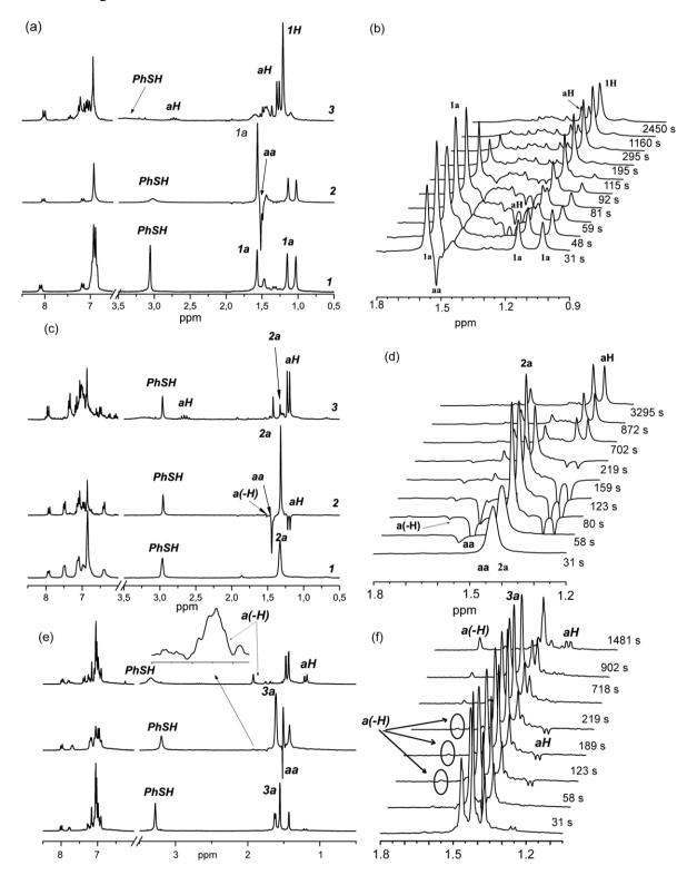
In the presence of radical scavenger, alkoxyamine is formed only as in-cage product of geminate radical pair RP, whereas escape radicals react with PhSH with the formation of alkane **aH**, hydroxylamine and other compounds. Thus, in this case CIDNP intensity of alkoxyamine is equal to the overall intensity of CIDNP of escape products, but with the opposite sign.
