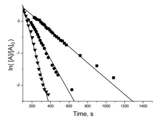
At time longer than 200 seconds, CIDNP kinetics are detected only on the protons of alkoxyamines and **aH**. The CIDNP kinetics decays of **1a–3a** at t > 200 s were described by monoexponential function with the decay parameter equal to  $k_{\rm obs}(T)$ . As an example Figure 4 shows CIDNP kinetics in logarithmic scale for **1a** providing  $k_{\rm obs}$  of  $2.0 \times 10^{-3}$  s<sup>-1</sup>,  $5.0 \times 10^{-3}$  s<sup>-1</sup>, and  $1.5 \times 10^{-2}$  s<sup>-1</sup>
