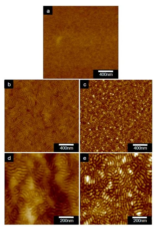
**Figure S2**. Height contrast AFM images of the surfaces of  $PS-b-PEO/SiO_2-TiO_2$  film containing (a) 10 vol% inorganic precursors; (b) 15 vol% inorganic precursors; (c) the identical film in (b) after removing the BCP templates; (d)  $PS-b-PEO/SiO_2-TiO_2$  film containing 20 vol% inorganic precursors; (e) identical film in (d) after removing the BCP templates. The hybrid films were prepared from spin coating dioxane solutions. Ti/Si mass ratio is 1.0.
