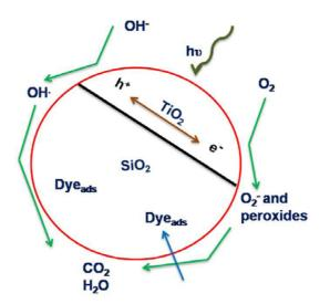
**Figure 7.** Electron transfer mechanism between dye and  $TiO_2$  with the role of  $SiO_2$ .
