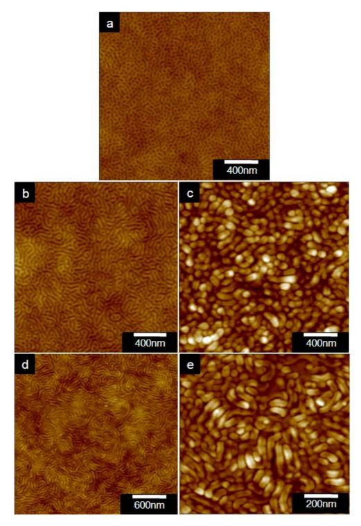
**Figure S3.** Height contrast AFM images of the surfaces of (a)  $PS-b-PEO/SiO_2-TiO_2$  film containing 10 vol% inorganic precursors; (b) identical film in (a) after removing the BCP templates; (c)  $PS-b-PEO/SiO_2-TiO_2$  film containing 20 vol% inorganic precursors; (d) identical film in (c) after removing the BCP templates. The hybrid films were prepared from spin coating dioxane solutions. Ti/Si mass ratio is 1.5.
