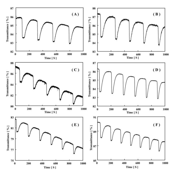
Figure 3 shows self-oscillating behaviors of the  $poly(VP-co-Ru(bpy)_3)$  solution in the different concentrations of malonic acid ([MA] = 0.04, 0.05, 0.06, 0.07, 0.08 and 0.09 M) under the fixed concentration of sodium bromate and nitric acid ([NaBrO<sub>3</sub>] = 0.3 M and [HNO<sub>3</sub>] = 0.3 M). As shown in Figure 3, the base line of the transmittance self-oscillation gradually decreased with time in all
