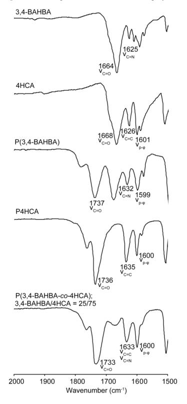
Figure 1. FT-IR spectra of the monomers and polymers.
