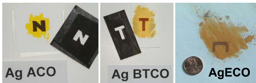
Figure 20. Practicality of color change upon exposure of Ag(I) cyanoximates to short-wavelength UV-radiation: potential for the battery-less colorimetric area detector for high-energy photons.
