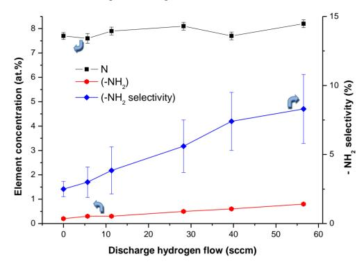
The treatment of 0.5 g of CNT-powder was thus carried out with the addition of 56.5 sccm of hydrogen gas in the post-discharge chamber. The CNTs were treated for 2 h using standard plasma parameters and, after their compression in pellet, they were derivatized with TFBA. XPS results are represented in Table 4.
