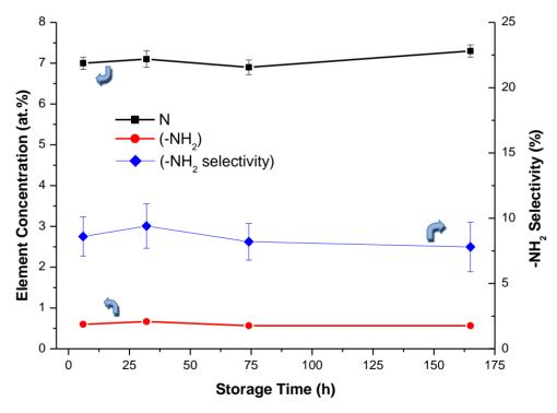
In order to take such stability into account, it may be suggested that primary amine functions could be stabilized by a delocalization of the nitrogen non-bonding electron pair into the aromatic rings of the graphene structure of the carbon nanotubes. This effect can be compared to the resonance delocalization observed in aniline.
