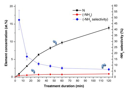
The results obtained after treatment of 0.5 g of the CNT powder are presented in Figure 7. In the case of the CNT powder treatment, the content in nitrogen and primary amines changes in the same proportion with the treatment time. The selectivity in grafted primary amines remains relatively high and constant at ca. 66%.
