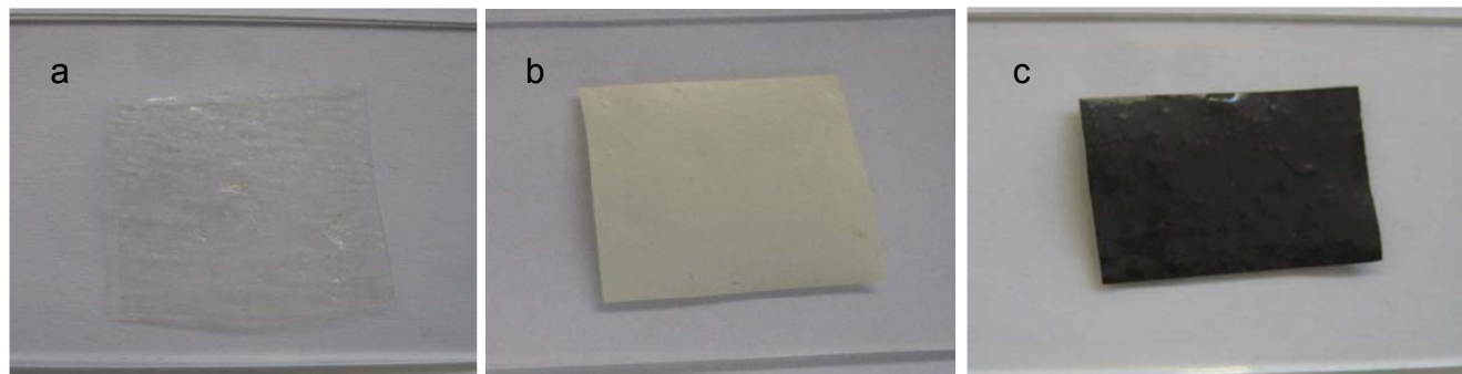
Figure 1. Optical images of typical films prepared by evaporative casting of (a) chitosan solution; (b) chitosan-TiO 2 dispersion; and (c) chitosan-Ag dispersion. Dimensions of films are 2.0 cm × 2.0 cm ((a) and (b)) and 3.0 cm × 2.0 cm (c). All films were prepared using chitosan batch CHM1.
