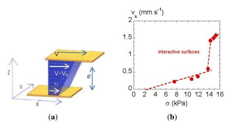
The apparent shear rate is:  $\dot{\gamma}_{app} = \frac{v}{e}$ , then  $\dot{\gamma}_{app} = \dot{\gamma} + \frac{2v_s}{e}$ . In this scheme, the sliding process is outlined by a no-zero velocity  $v_s$  with respect to the walls (Figure 5(a)). The sliding velocity,  $v_s$  can be
