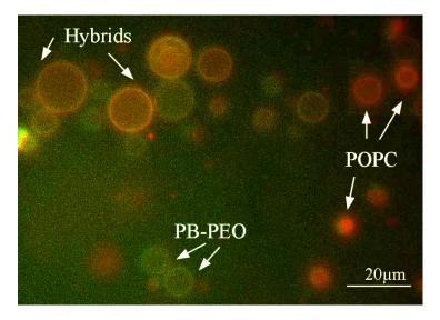
Importantly, our results show that both nanometer-sized and micrometer-sized hybrid vesicles can be formed when employing low molecular weight PB-PEO polymers that more closely match the dimensions of phospholipids.
