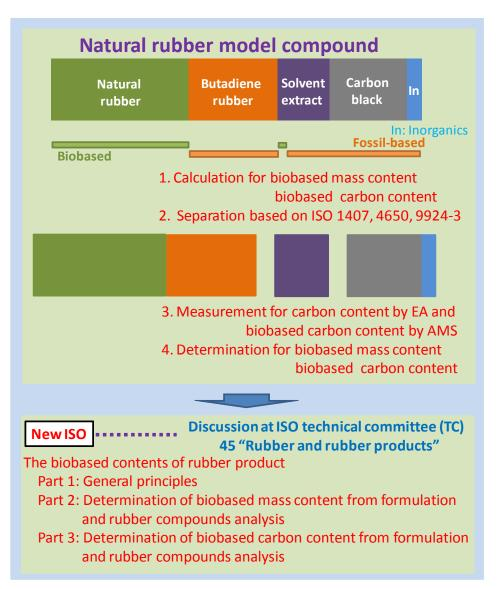
Figure 8. Determination methods of biobased contents for ISO evaluation methods.
