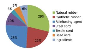
Figure 1. Composition of main materials used in automobile tires in Japan in 2012 [5].
