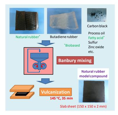
Figure 3. Production of natural rubber model compound.
