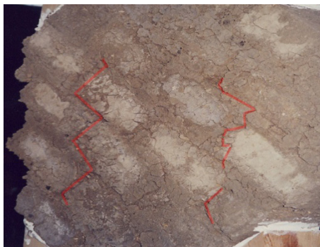
Figure 5. Detail of the experimental crack pattern (unreinforced plain adobe soil) (reprinted with permission from [7], Copyright 2001 Elsevier).
