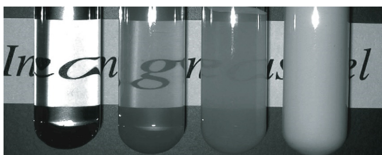
Figure 1. The appearance of the opaque poly(acrylamide) gels. The mole fraction of the cross-linker is 0.01, 0.03, 0.05 and 0.1 from left to right. The total concentration of the pre-gel solution is fixed at 700 mM.
