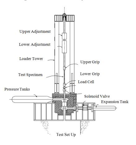
Figure 4. Schematic 890 kN Dynamic Loader.
