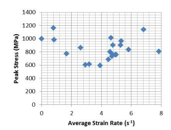
Figure 7. Peak stress vs. average strain rate for all coupons.
