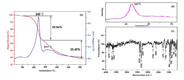
**Figure 7.** (a) TGA and DTG curves of PVTNP-*g*- $3^{\#}$ GAP under nitrogen; (b) The thermal decomposition gas intensity under different temperature; (c) The IR spectrum of the thermal decomposition gas of PVTNP-*g*- $3^{\#}$ GAP at 240 °C under nitrogen.
