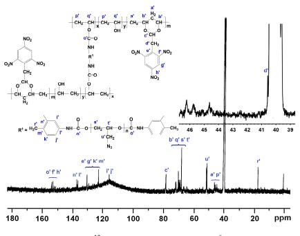
Figure 4. <sup>13</sup>C NMR spectrum of PVTNP-g-3<sup>#</sup>GAP.
