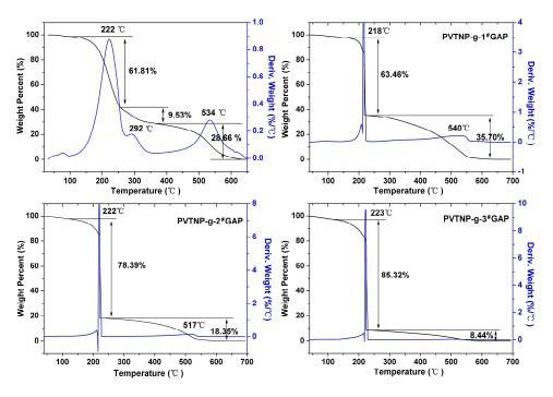
Figure 6. The TGA and DTG curves of PVTNP and PVTNP-g-GAPs under air atmosphere.
