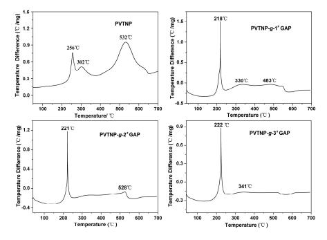
Figure 5. The DTA curves of PVTNP and PVTNP-g-GAPs under air atmosphere.
