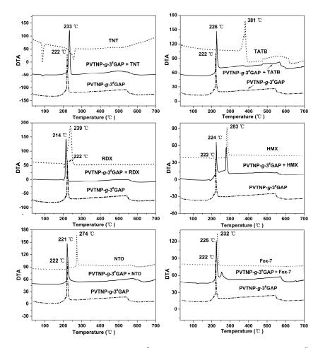
**Figure 9.** DTA curves of PVTNP-*g*-3<sup>#</sup>GAP and a mixture of PVTNP-*g*-3<sup>#</sup>GAP/TNT, PVTNP-*g*-3<sup>#</sup>GAP/TATB, PVTNP-*g*-3<sup>#</sup>GAP/RDX PVTNP-*g*-3<sup>#</sup>GAP/HMX, PVTNP-*g*-3<sup>#</sup>GAP/NTO and PVTNP-*g*-3<sup>#</sup>GAP/FOX-7.
