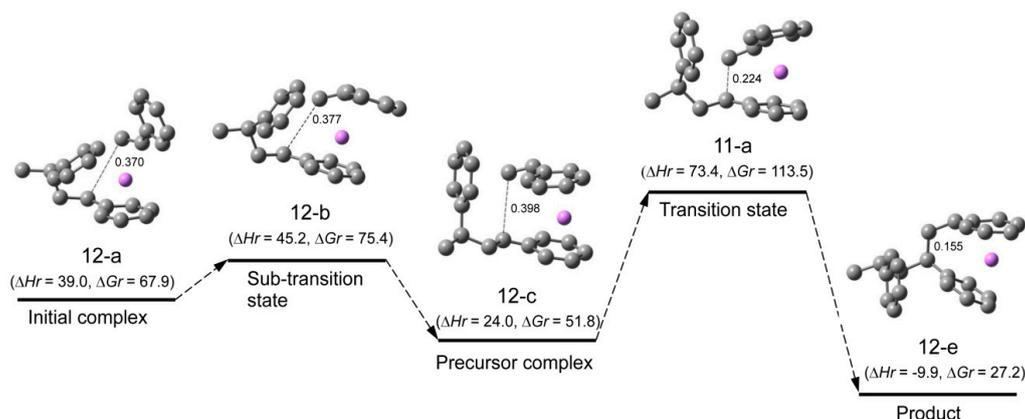
**Figure 12.** Reaction pathway for system(s-11-a) (St/[HSt<sub>2</sub>Li(10-c)]) in the gas phase.  $\Delta H_r$  and  $\Delta G_r$ , the relative enthalpy and relative free energy, are expressed in kJ·mol<sup>-1</sup>. Hydrogen atoms are not shown. Numerical values in the drawings as in Figure 5.
