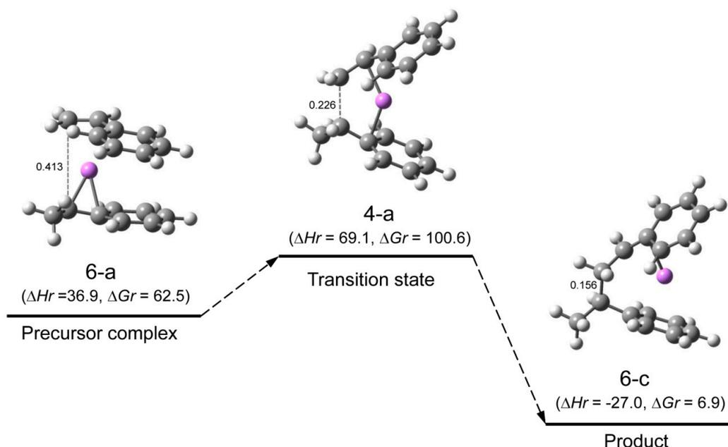
**Figure 6.** Reaction pathway for system(s-4-a) (St/[HStLi(2-a)]) in the gas phase.  $\Delta H_r$  and  $\Delta G_r$ , the relative enthalpy and relative free energy, are expressed in kJ·mol<sup>-1</sup>. Numerical values in the drawings as in Figure 5.
