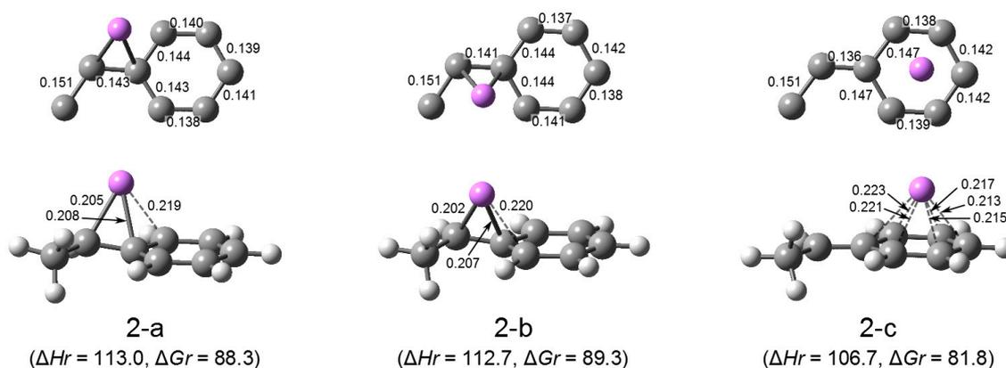
**Figure 2-1.** Optimized geometries and relative energies of HStLi in the gas phase. The small drawing on the upper part of each structure is the simplified overhead view of the lower drawing. C–Li distances less than 0.225 nm are shown in the lower drawings, and C–C bond distances are shown in the upper drawings. Δ*Hr* and Δ*Gr*, the relative enthalpy and relative free energy, are expressed in kJ·mol<sup>-1</sup>.
