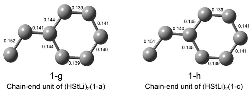
**Figure 1-2.** C–C bond distances of  $(\text{HStLi})_2(1-a)$  and  $(1-c)$ . Geometry of the carbon framework of one chain-end unit (HSt-) is shown for  $(\text{HStLi})_2(1-a)$  and  $(1-c)$ . Distances of C–C bonds are expressed in nm.
