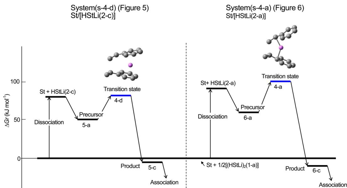
**Figure 8.** Free energy changes for the addition of styrene to HStLi in the gas phase.
