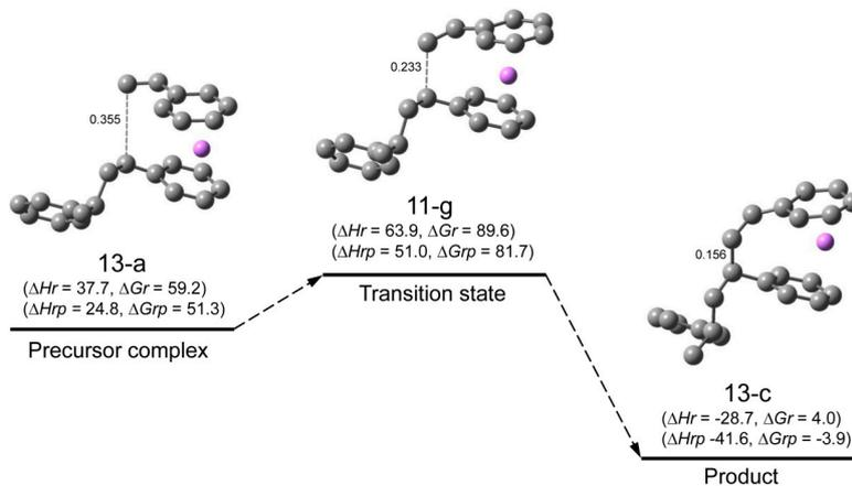
**Figure 13.** Reaction pathway for system(s-11-g) (St/[HSt<sub>2</sub>Li(10-f)]) in the gas phase.  $\Delta H_r$  and  $\Delta G_r$ , the relative enthalpy and relative free energy, are expressed in kJ·mol<sup>-1</sup>.  $\Delta H_{rp}$  and  $\Delta G_{rp}$  in the lower parentheses are the enthalpy and free energy with respect to (St + 1/2[(HSt<sub>2</sub>Li)<sub>2</sub>(9-f)]), in kJ·mol<sup>-1</sup>. The other drawing details as in Figure 12.
