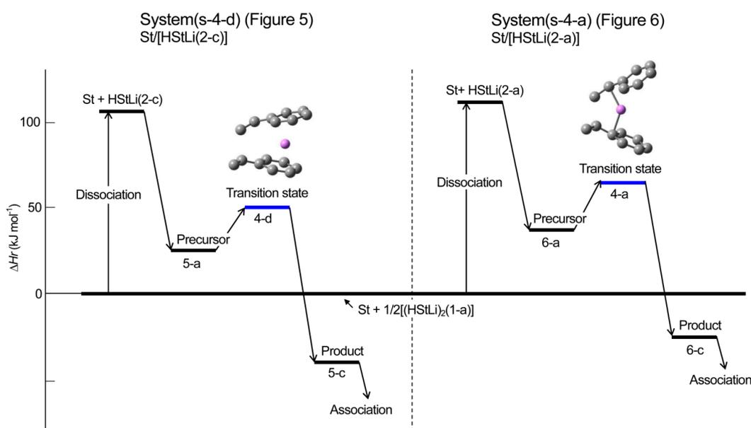
**Figure 7.** Enthalpy changes for the addition of styrene to HStLi in the gas phase.
