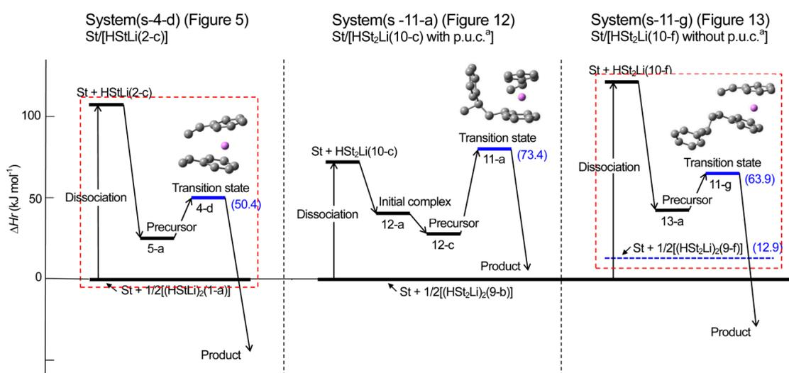
**Figure 14.** Enthalpy changes for the addition of styrene to  $\text{HStLi}$  and  $\text{HSt}_2\text{Li}$  in the gas phase. The sub-transition state between the initial complex and the precursor for system(s-11-a) is not shown here. <sup>a</sup> p.u.c.: penultimate unit coordination.
