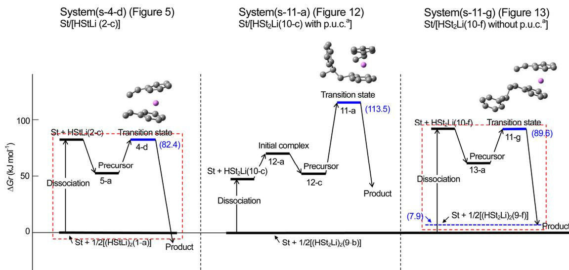
**Figure 15.** Free energy changes for the addition of styrene to HStLi and HSt<sub>2</sub>Li in the gas phase. The sub-transition state between the initial complex and the precursor for system(s-11-a) is not shown here. <sup>a</sup> p.u.c: penultimate unit coordination.
