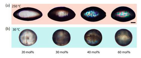
**Figure 4.** Shape transformation of LCE particles in the temperature range of 30 °C (**b**) and 250 °C (**a**). The particles contain different amounts of the liquid crystalline diacrylate crosslinker and were synthesized under the same microfluidic conditions (images were taken between crossed polarizers, scale bar: 100  $\mu$ m).
