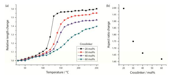
**Figure 5.** (a) Phase behavior of LCE particles, which contain different crosslinker densities. The relative length change along the particles' long axis  $l(T)/l(30 \degree C)$  is illustrated as a function of the temperature; (b) Change of the LCE particles' aspect ratio AR(250 °C)/AR(30 °C) as dependent on the crosslinker density.
