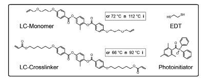
**Figure 2.** Chemical structures of the components which were used in the liquid crystalline monomer mixture. The phase transition temperatures of the mesogenic LC-monomer and LC-crosslinker were measured via differential scanning calorimetry. (EDT: 1,2-ethanedithiol).
