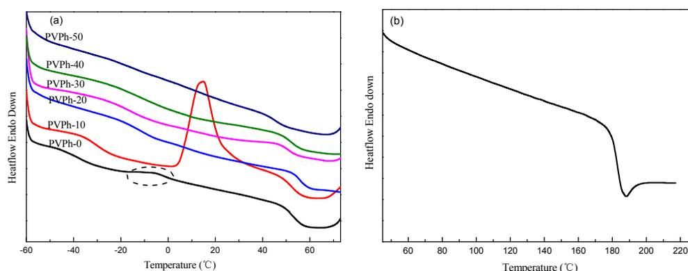
**Figure 2.** Differential scanning calorimetry (DSC) heating curves for melt-quenched (a) PBSA/PVPh/PLLA blends and (b) PVPh at a rate of 10 °C/min.
