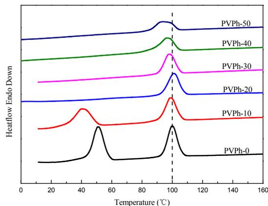
**Figure 4.** Non-isothermal crystallization DSC curves for PBSA/PVPh/PLLA blends.
