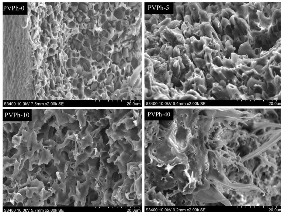
**Figure 3.** Scanning Electron Microscope (SEM) micrographs for PBSA/PVPh/PLLA fracture surfaces after being etched with tetrahydrofuran.
