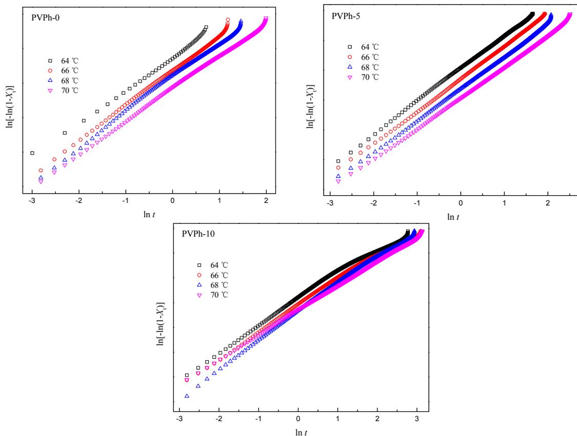
Figure 5. Avrami plots for PBSA isothermally crystallization in blend samples.
