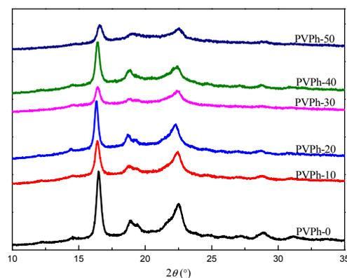
Figure 7. WAXD patterns for PBSA/PVPh/PLLA blend samples.
