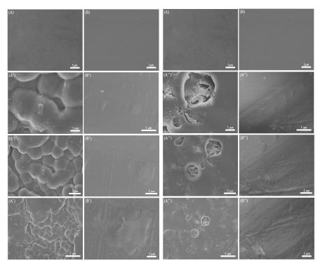
**Figure 5.** SEM images of novel PAI and pure PAI after 1, 3 days degradation at 37 °C in PBS. Before degradation ((**A**) novel PAI; (**B**) pure PAI); After degradation for 1 day ((**A**') novel PAI; (**B**') pure PAI); After degradation for 3 days ((**A**'') novel PAI; (**B**'') pure PAI).
