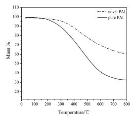
Figure 3. TGA thermograms of novel PAI and pure PAI.
