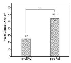
**Figure 4.** The water contact angle of the novel PAI and the pure PAI (\*\* p < 0.01).
