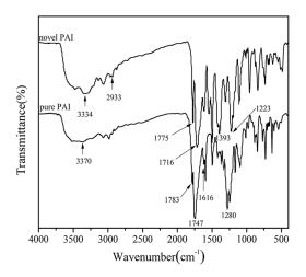
Figure 1. FTIR spectra of novel PAI and pure PAI.
