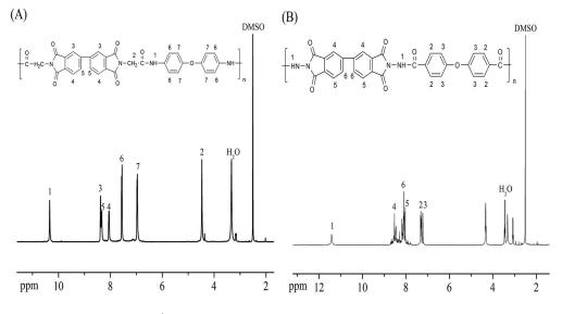
**Figure 2.** <sup>1</sup>H NMR spectra of novel PAI (**A**) and pure PAI (**B**).
