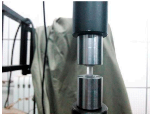
Figure 3. The fixture device connecting the specimen in quasi-static tension tests.
