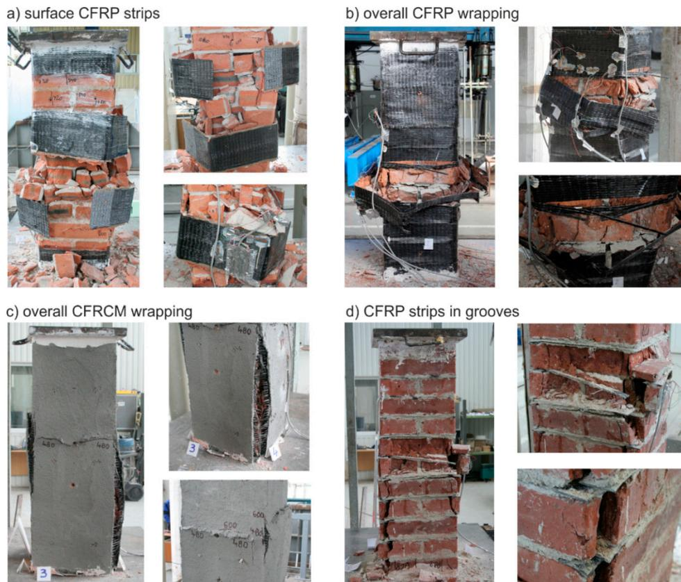
**Figure 9.** Characteristic failures of reinforced brick masonry columns at reaching ultimate load; (a) CFRP strips on surface (EBR); (b) overall CFRP wrapping; (c) overall CFRCM wrapping; (d) CFRP pre-laminated strips inserted into grooves (NSM).
