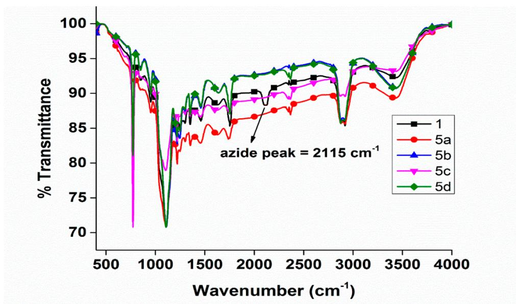
Figure S6. IR spectra of polymers (1 and 5a–5d).
