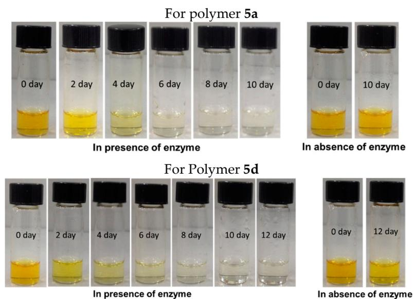
**Figure S13.** Time dependent release of curcumin from polymers 5a and 5d, with/without incubation of enzyme.
