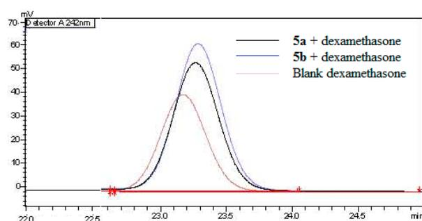
Figure S16. HPLC chromatogram of dexamethasone encapsulated in fluorinated polymeric samples using acetonitrile:water:phosphoric acid (30:70:0.5, v/v/v) as an eluent.
