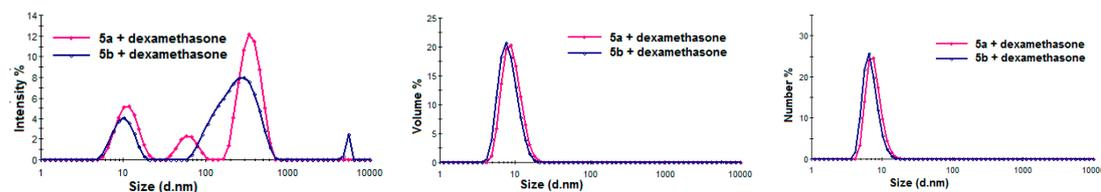
Figure S9. DLS size distribution graphs of dexamethasone encapsulated polymers 5a and 5b.
