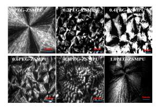
Figure 4. Polarized optical microscope (POM) images (magnified 100 times) of PEG-ZSMPUs.
