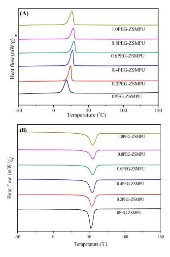
**Figure 7.** Differential scanning calorimeter (DSC) curves of PEG-ZSMPUs: (**A**) the cooling curves and (**B**) the second DSC heating curves.
