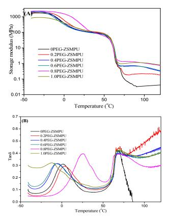
**Figure 9.** The Dynamic mechanical analysis (DMA) curves of PEG-ZSMPUs (**A**) storage modulus and (**B**) tan  $\delta$  curves.
