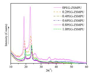
Figure 3. X-ray diffractometry (XRD) curves for PEG-ZSMPUs.
