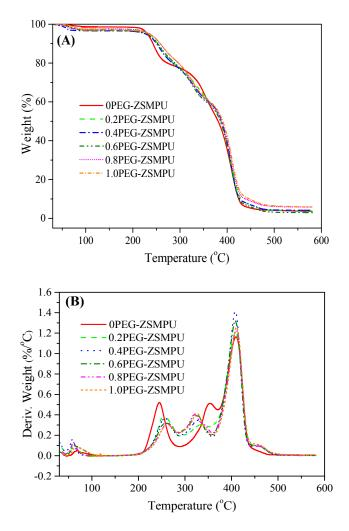
**Figure 8.** Thermogravimetric analysis (TGA curves of PEG-ZSMPUs: (**A**) TG curves, and (**B**) DTG curves).
