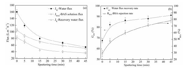
**Figure 5.** Permeation separation performance (including pure water flux, recovery flux, BSA solution flux, water flux recovery rate, and BSA rejection rate) of the metalized membranes with different sputtering times.
