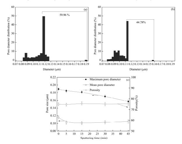
**Figure 4.** Pore diameter distribution of (**a**) M0 and (**b**) M45 and the (**c**) porosity, maximum pore diameter, and mean pore diameter of the metalized membranes with different sputtering times.
