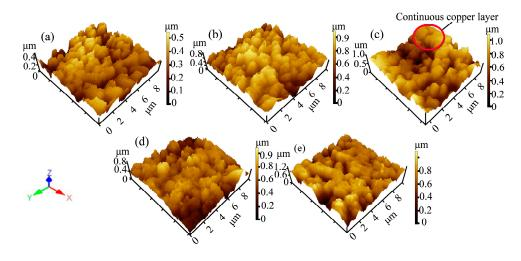
**Figure 1.** AFM images of the metalized membranes (10  $\mu$ m × 10  $\mu$ m) with different sputtering times: (a) M0; (b) M5; (c) M15; (d) M30; and (e) M45.
