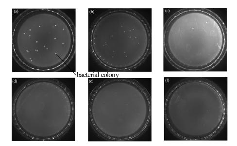
**Figure 6.** Media photos that correspond to the sample membranes with antibacterial properties under different sputtering times. (a) Blank control group; (b) virgin membranes; (c) 5 min; (d) 15 min; (e) 30 min; and (f) 45 min.
