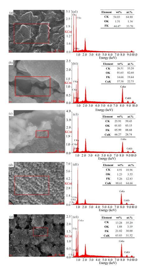
**Figure 3.** Chemical elemental composition measured using EDX for M0 (**a**,**a**1), M15 (**b**,**b**1,**c**,**c**1), and M45 (**d**,**d**1,**e**,**e**1): (**a**,**b**,**d**) surface morphology, (**a**1,**b**1,**d**1) elements on the surface, (**c**,**e**) cross-section morphology, and (**c**1,**e**1) elements at the cross-section near the surface.
