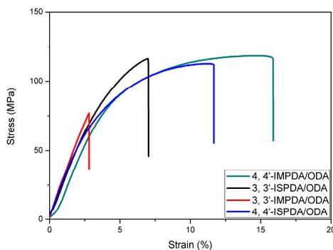
Figure 7. Representative stress-strain curves of isohexides-derived PEIs.
