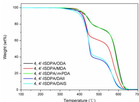
**Figure 5.** Representative TGA traces of isohexide-derived poly(ether imide)s (PEIs).
