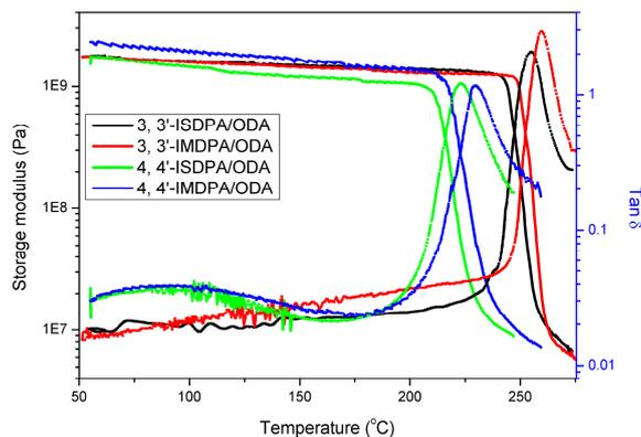
Figure 6. Representative DMTA curves of isohexides-derived PEIs.
