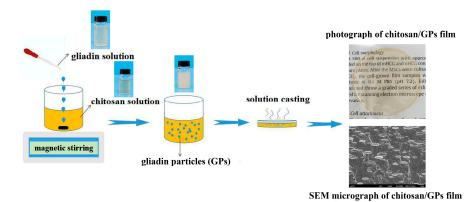
Figure 1. Schematic of fabrication mechanism of chitosan/gliadin particles (CS/GPs) biocomposites.
