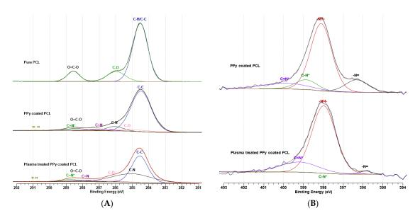
**Figure 5.** High-resolution XPS spectra of the coated and uncoated samples at C 1 s, and comparison of the coated samples without and with plasma treatment at N 1 s. (**A**) High-resolution C 1 s spectrum for PCL and PPy-coated PCL fibers without and with plasma treatment; (**B**) High-resolution N 1 s spectrum for PPy-coated PCL fibers without and with plasma treatment.
