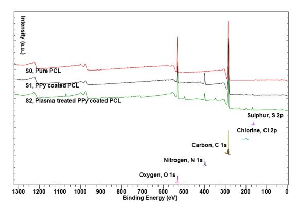
**Figure 4.** XPS wide spectra for PCL, PPy-coated PCL without and with plasma treatment. Nitrogen, chlorine and sulphur peaks are available for the coated samples. There is some contamination of plasma-treated sample, which is expected to be due to the contamination of the plasma chamber.
