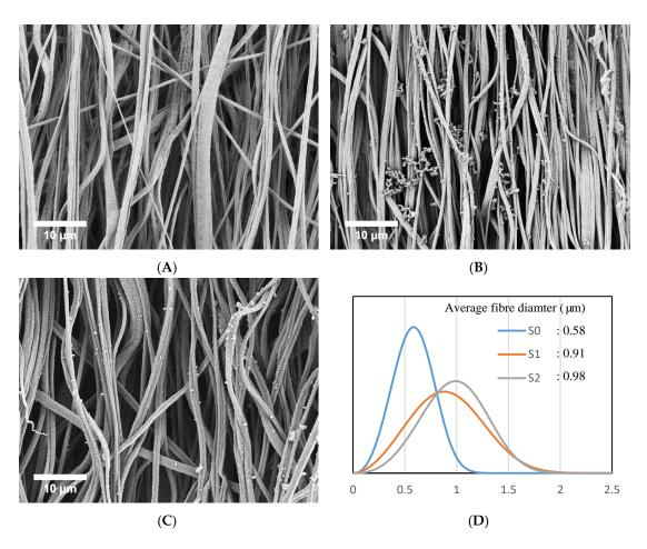
**Figure 2.** The morphology of the fibers and the fiber diameter distribution. **(A)** Aligned PCL fibers without coating (S0); **(B)** Aligned PPy-coated PCL fibers (S1); **(C)** Plasma-treated aligned PPy-coated PCL fibers (S2); **(D)** Fiber diameter distribution by Weibull curve fitting.
