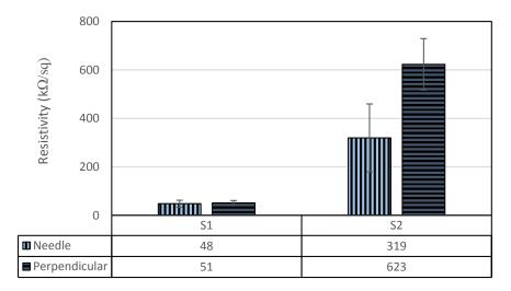
**Figure 6.** The electrical resistivity of the PPy-coated PCL fibers without (S1) and with plasma treatment (S2). The plasma treatment formed the more stable bond  $C=N^+$ , which replaced the bonds with high electron freedom,  $C-N^+$  and -N=.
