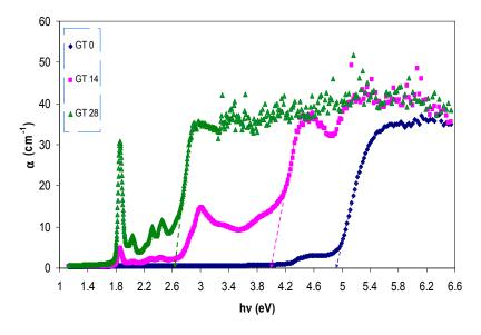
Figure 7. The absorption coefficients versus photon energy for pure PMMA and PMMA doped samples.
