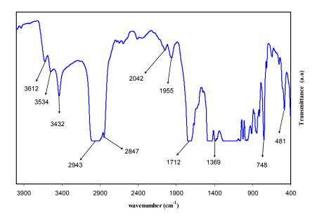
**Figure 4.** FTIR spectra of dye doped PMMA polymer (GT 28). Shifting of peaks and their broadening is evidence for the complex formation between the extract GT solution and PMMA polymer.
