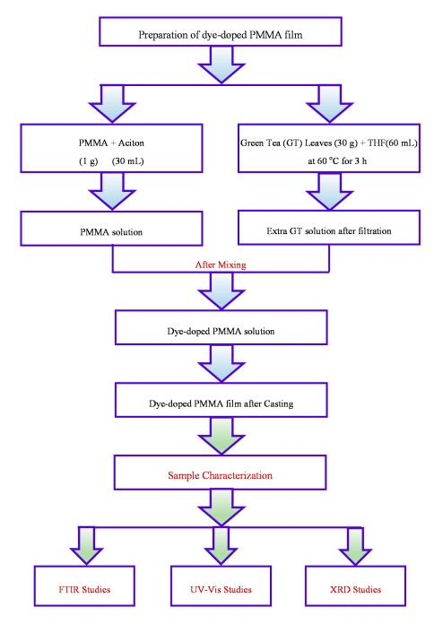
Figure 1. Flowchart of the experimental method and characterization techniques.
