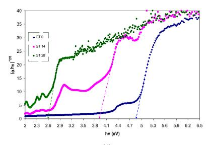
**Figure 10.** The plots of  $(\alpha hv)^{2/3}$  vs. (*hv*) for all the samples.
