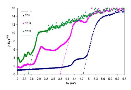
**Figure 9.** The plots of  $(\alpha hv)^{1/2}$  vs. (*hv*) for all the samples.
