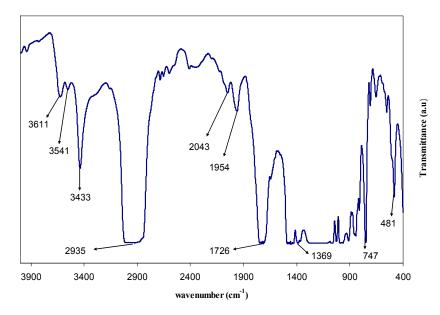
**Figure 3.** FTIR spectra of pure PMMA polymer (GT 0). It is obvious that the peaks are sharp and their intensity is high.
