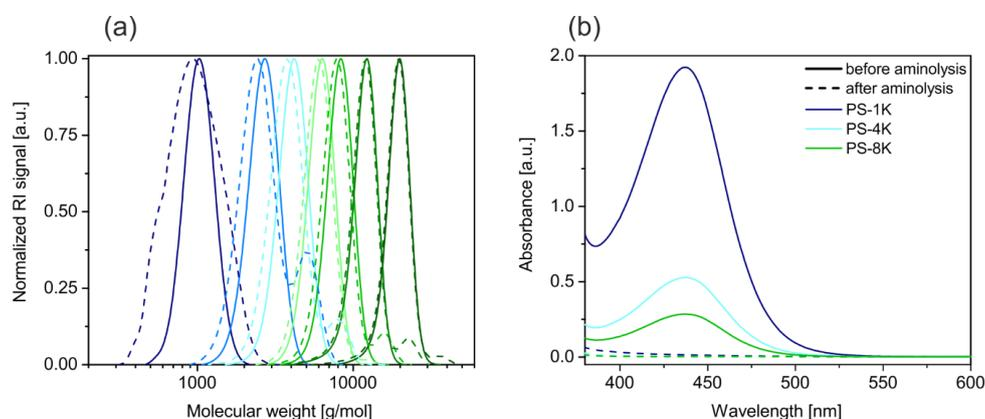
**Figure 2.** (a) Molecular weight distributions of the polystyrene ligands before (solid lines) and after (dashed lines) the aminolysis. (b) UV-VIS spectra of the 1 K, 4 K, and 8 K ligands before (solid lines) and after (dashed lines) the aminolysis. The absence of the  $n \rightarrow \pi^*$  transition proves the successful reaction. The absorbance decreases with increasing molecular weight, which correlates well to the ratio between trithiocarbonate end-groups and the ligand length.
