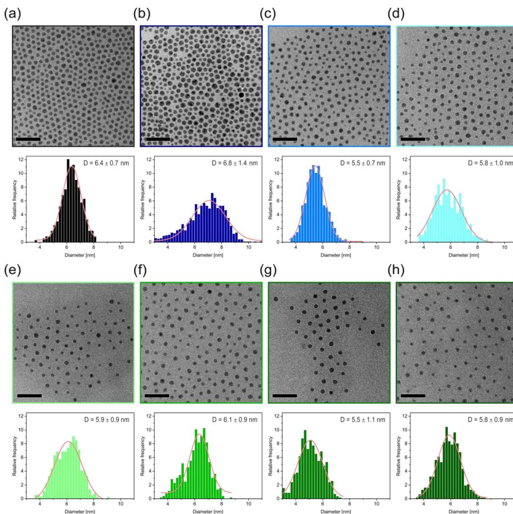
**Figure 4.** (a) Pure Ag@myristate nanoparticles. (b–h) nanocomposite samples with the following molecular weight of the polystyrene ligands: (b) 1 kg/mol; (c) 3 kg/mol; (d) 4 kg/mol; (e) 6 kg/mol; (f) 8 kg/mol; (g) 12 kg/mol; and (h) 18 kg/mol. The interparticle distance increases with increasing molecular weight. All scale bars are 50 nm. The histograms in the bottom panel show the size distributions of the Ag core diameter of the respective sample.
