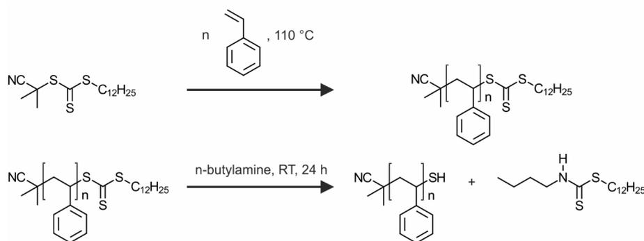
**Figure 1.** Reaction scheme of the RAFT polymerization (**top**) and the aminolysis to yield a thiol functionalization (**bottom**).
