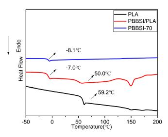
Figure 8. DSC curves of the PBBSI/PLA TPV and its individual components.
