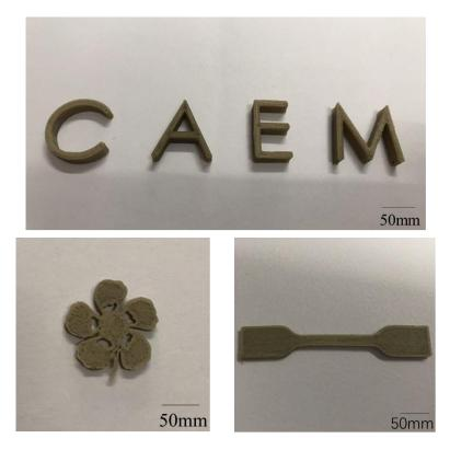
Figure 12. 3D-printed samples of the PBBSI/PLA TPV.
