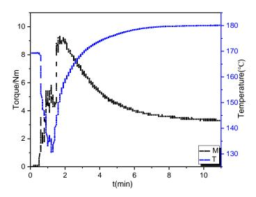
Figure 6. Dynamical vulcanization curves of PBBSI copolyesters.
