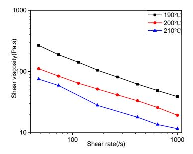
Figure 11. Rheological curves of the PBBSI/PLA TPV.
