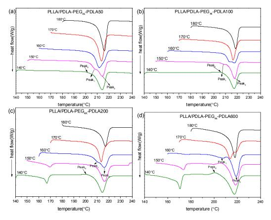
**Figure 10.** DSC heating curves of PLLA/PDLA-PEG<sub>4k</sub>-PDLA with different PDLA blocks isothermally crystallized at different temperatures: (a) PLLA/PDLA-PEG<sub>4k</sub>-PDLA50; (b) PLLA/PDLA-PEG<sub>4k</sub>-PDLA100; (c) PLLA/PDLA-PEG<sub>4k</sub>-PDLA200; (d) PLLA/PDLA-PEG<sub>4k</sub>-PDLA600.
