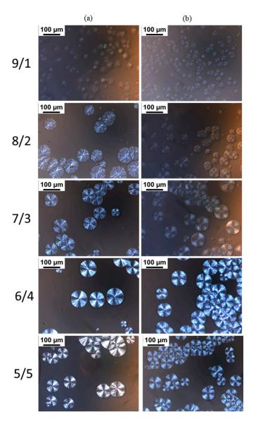
**Figure 4.** Polarizing optical microscopy (POM) images of the blends with different L/D ratios isothermally crystallized at 160 °C: (a) PLLA/PDLA-PEG<sub>1k</sub>-PDLA100; (b) PLLA/PDLA-PEG<sub>4k</sub>-PDLA400.
