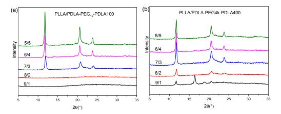
**Figure 3.** X-ray diffraction (XRD) curves of PLLA/PDLA-PEG<sub>1k</sub>-PDLA100 (**a**) and PLLA/PDLA-PEG<sub>4k</sub>-PDLA400 (**b**) with different L/D ratios (Each sample was first melted at 240  $^{\circ}$ C for 4 min and then cooled to room temperature at 10  $^{\circ}$ C/min).
