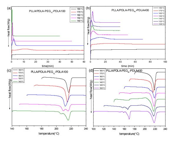
**Figure 6.** DSC curves of isothermal crystallization process (a,b) at different temperatures and subsequently heating processes (c,d): (a,c) PLLA/PDLA-PEG<sub>1k</sub>-PDLA100 and (b,d) PLLA/PDLA-PEG<sub>4k</sub>-PDLA400.
