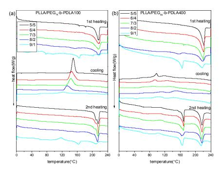
**Figure 2.** Differential scanning calorimetry (DSC) curves of PLLA/PDLA-PEG<sub>1k</sub>-PDLA100 (**a**) and PLLA/PDLA-PEG<sub>4k</sub>-PDLA400 (**b**) with different L/D ratios.
