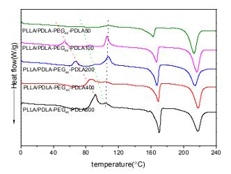
**Figure 7.** DSC heating curves of PLLA/PDLA-PEG $_{4k}$ -PDLA blends with different PDLA blocks after quenching from 240  $^{\circ}$ C.
