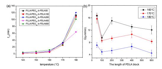
**Figure 8.** (a) Crystallization half-time  $(t_{1/2})$  and (b) radial growth rate of spherulites of (*G*) of PLLA/PDLA-PEG<sub>4k</sub>-PDLA with different PDLA blocks isothermally crystallized at different temperatures.
