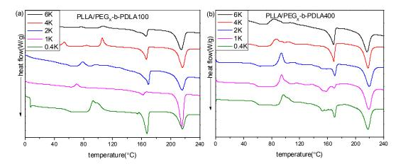
**Figure 5.** DSC heating curves of blends with different PEG blocks after quenching from 240 °C: (a) PLLA/PDLA-PEG<sub>1k</sub>-PDLA100; (b) PLLA/PDLA-PEG<sub>4k</sub>-PDLA400.
