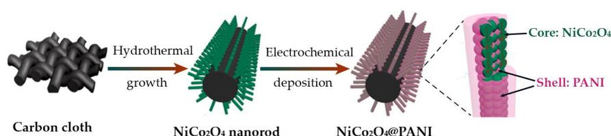
**Figure 14.** Schematic of the synthetic procedure for NiCo<sub>2</sub>O<sub>4</sub>@PANI nanorod arrays. Reprinted with permission from [134]. Copyright 2016, American Chemical Society.
