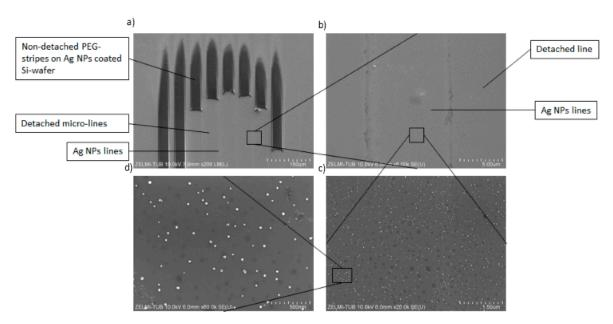
Figure S2. (a–d) SEM images of the micro-patterned Ag NPs on SI-wafer using wet μ-CdP approach.
