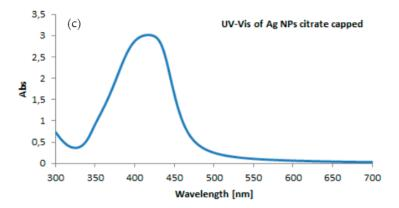
**Figure S1**. (**a**,**b**) AFM height images and cross section profiles and (**c**) UV-Vis spectrum of citrate capped Ag NPs.
