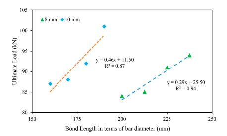
Figure 14. Relationship between the bond length and ultimate load carrying capacity.
