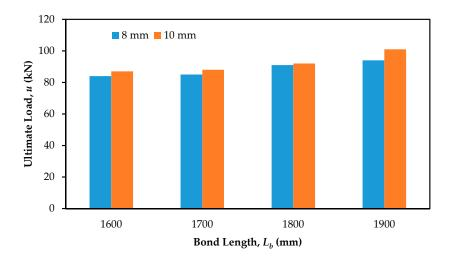
Figure 13. The effect of bond length on the ultimate load.
