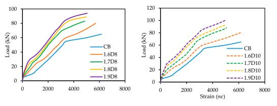
(a) For 8-mm Ø strengthened specimens
