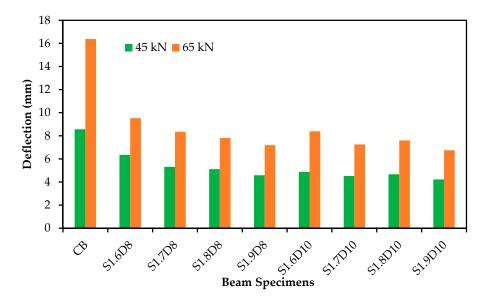
Figure 7. Deflection at different loads (45 and 65 kN).
