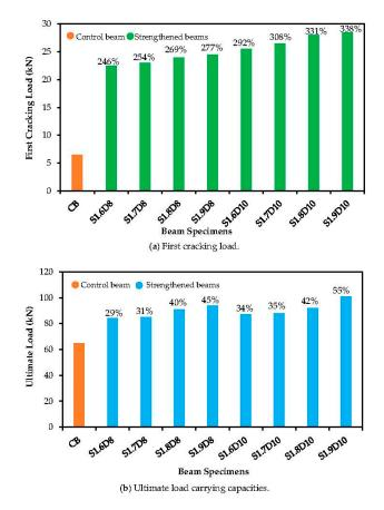
Figure 5. Flexural capacities improved by SNSM-GFRP bars.
