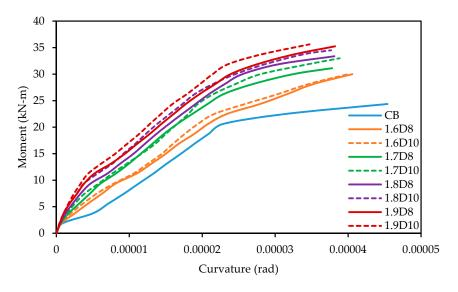
Figure 18. Moment-curvature relationship for all beam specimens.
