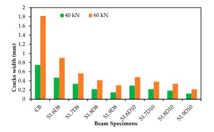
Figure 9. Cracks width of the specimens at 40 and 60 KN.
