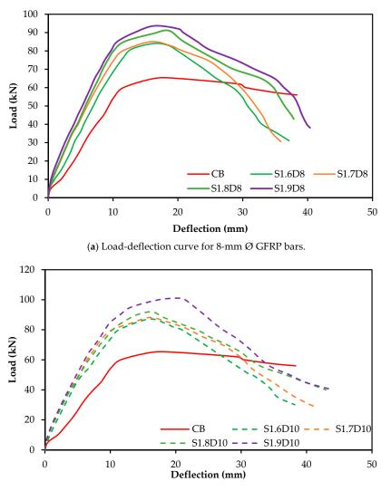
(b) Load-deflection curve for 10-mm Ø GFRP bars.
