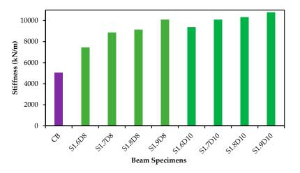
Figure 12. Stiffness of the beam specimens.
