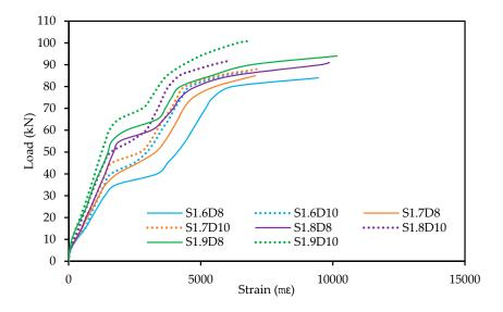
Figure 17. Tensile strain in the SNSM-GFRP bars.
