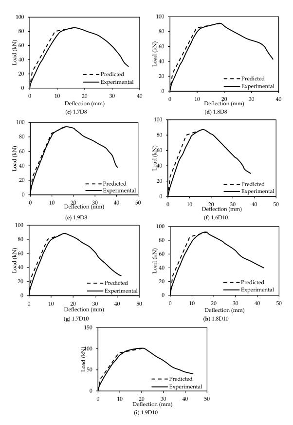
Figure 19. Comparison between the experimental and predicted load-deflection curves.
