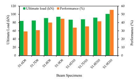
Figure 15. The effect of strengthening reinforcements on the flexural performance.
