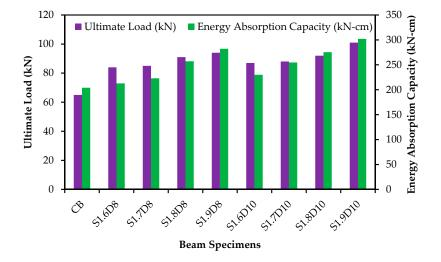
Figure 11. Ultimate load and energy absorption capacities of the specimens.
