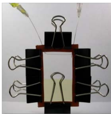
Figure S2. The liquid/liquid procedure where both pre-polymer solutions were injected sequentially into the mold. The bottom layer in yellow is the DMAEMA layer in water, the transparent layer on the top is the BMA layer in toluene.
