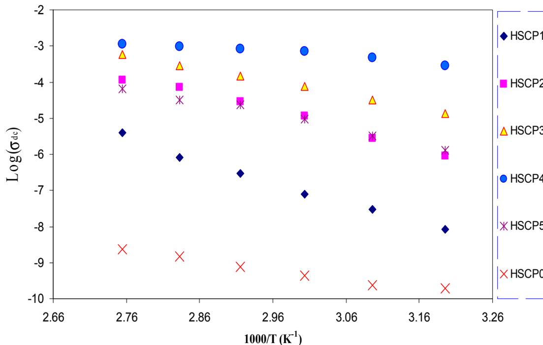
Figure 5. Temperature dependence of DC ionic conductivity for all samples.
