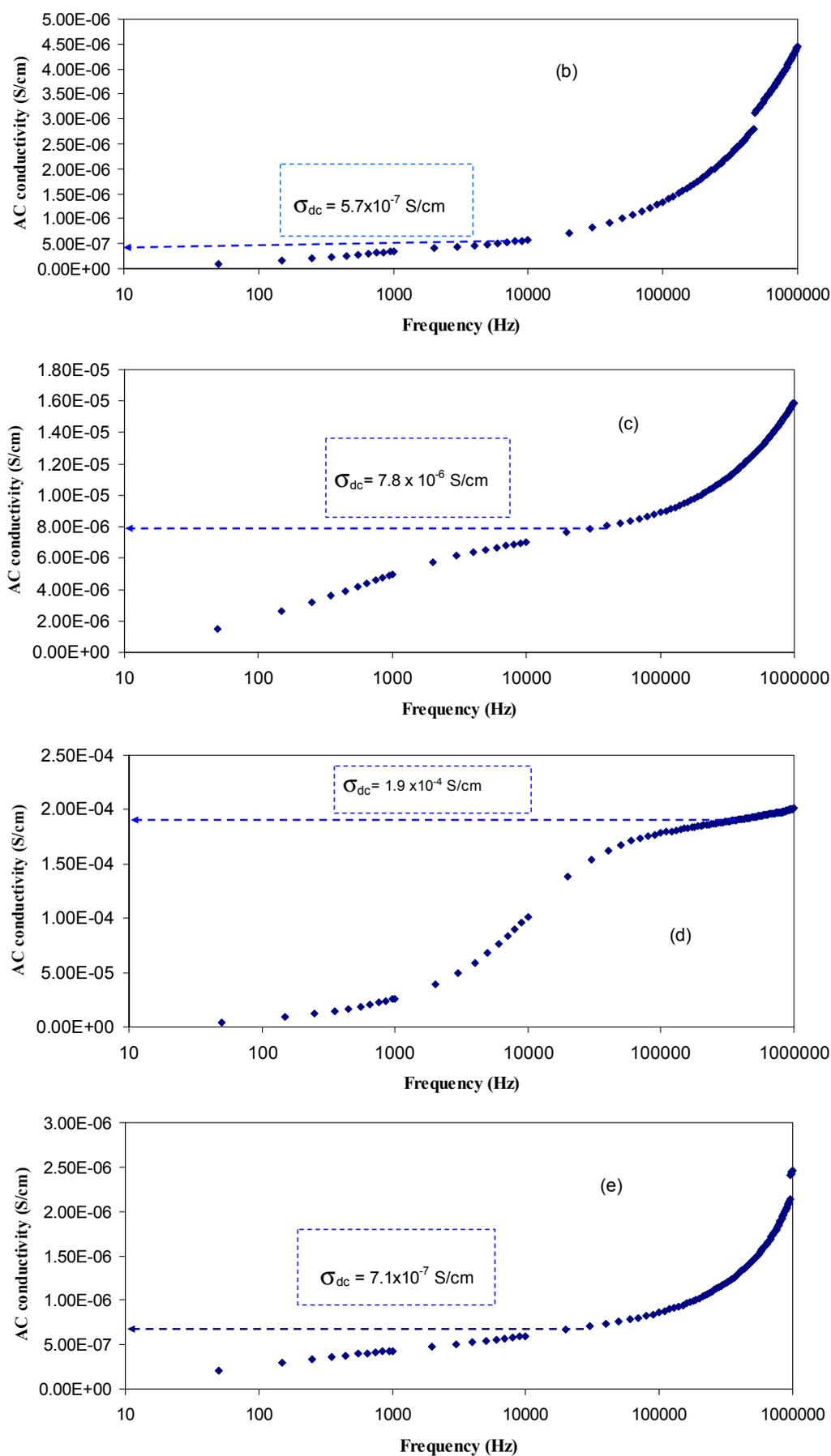
Figure 7. AC conductivity spectra for (a) HSCP 1; (b) HSCP 2; (c) HSCP 3; (d) HSCP 4 and (e) HSCP 5.
