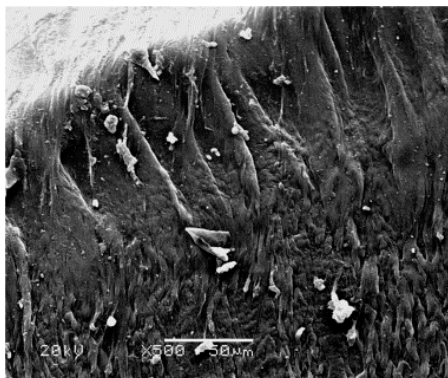
Figure 6. SEM image of the craze-shearing zone shown in Figure 5.
