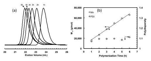
**Figure 3.** (a) GPC elution curves for polyethylene samples taken at different polymerization time in ethylene polymerization using **2** at 5 °C and 400 psi in chlorobenzene; and (b) plot of  $M_n$  and *PDI* as functions of polymerization time.
