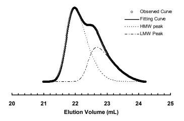
Figure 5. Deconvolution of GPC elution curve for sample 3b-E400-3.
