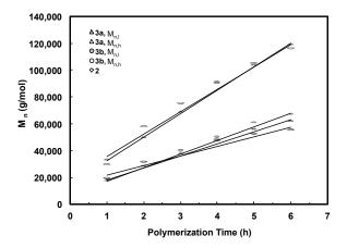
**Figure 7.** Number-average molecular weight of deconvoluted peaks as a function of polymerization time for polymers produced with catalyst **3a** and **3b** under 5 °C and 400 psi. Comparison is made with polymers prepared using catalyst **2**.
