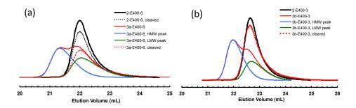
**Figure 9.** Comparison of GPC elution curves of polymer samples before and after cleavage: (**a**) samples 2-E400-6 and 3a-E400-6; and (**b**) samples 2-E400-3 and 3b-E400-3.
