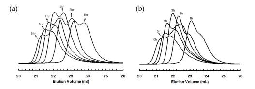
**Figure 4.** GPC elution curves for polyethylene samples taken at different polymerization time in ethylene "living" polymerization using (**a**) **3a**; and (**b**) **3b**, at 5 °C and 400 psi in cholorobenzene.
