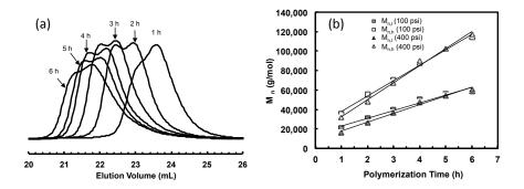
**Figure 10.** (a) GPC elution curves for polyethylene samples taken at different polymerization time in ethylene polymerization using **3a** at 5 °C and 100 psi in chlorobenzene; and (b)  $M_{n,l}$  and  $M_{n,h}$  values of the deconvoluted peaks as a function of polymerization time for polymers produced at 100 psi and 400 psi using **3a**.
