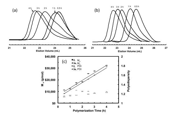
**Figure 11.** GPC elution curves of poly(1-hexene)s produced at different polymerization time using: (a) **2**; and (b) **3a**, at 0 °C and [1-hexene] = 1.15 M. (c) Plot of  $M_n$  and *PDI* for poly(1-hexene)s produced with **2** and **3a** as functions of polymerization time.
