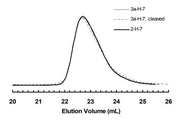
Figure 12. GPC elution curve of cleaved sample 3a-H-7, in comparison with those of 3a-H-7 and 2-H-7.
