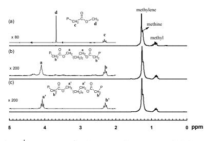
**Figure 8.** Polymer <sup>1</sup>H NMR spectra for: (**a**) 2-E400-2; (**b**) 3a-E400-2; and (**c**) 3b-E400-2. All three polymers were produced after 2 h of polymerization time.
