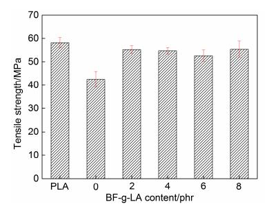
Figure 5. Tensile strength of PLA/BF/BF-g-LA composites.
