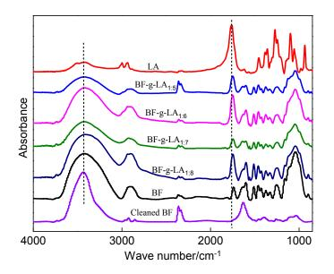
Figure 2. Infrared spectra of BF-g-LA.
