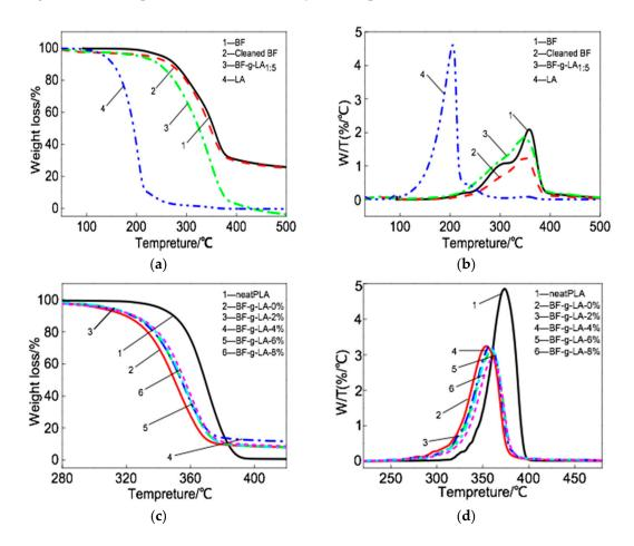
**Figure 4.** Thermal weightlessness curve for BF-*g*-LA and PLA/ BF/B-*g*-LA composites (**a**) TG curve for BF-*g*-LA; (**b**) DTG curve for BF-*g*-LA; (**c**) TG curves for PLA/BF/BF-*g*-LA composites; (**d**) DTG curve for PLA/BF/BF-*g*-LA composites.
