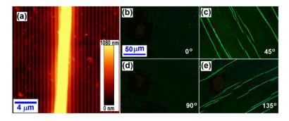
**Figure 2.** (a) AFM image measured on the F8BT fibers prepared on a photoresist grating template; and (**b–e**) polarization optical microscopic images of the F8BT fibers.
