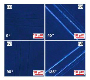
**Figure 4.** Polarization optical microscopic images measured on the PFB fibers with the grating lines orientated at (a)  $0^{\circ}$ ; (b)  $45^{\circ}$ ; (c)  $90^{\circ}$ ; and (d)  $135^{\circ}$  with respect to one of the two orthogonally-arranged polarizers.
