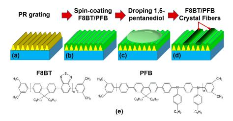
**Figure 1.** Fabrication procedures for the F8BT fibers. (a) The template PR grating with a period of 670 nm on a glass substrate; (b) spin-coating of the polymer film; (c) drop casting of 1,5-pentanediol onto the top surface of the polymer film; (d) growth of the polymeric fibers; and (e) chemical structures of F8BT and PFB.
