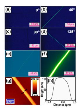
**Figure 3.** (**a**–**d**) Polarization optical microscopic images of a single F8BT fiber; (**e**,**f**) transmission and fluorescence optical microscopic image of the single F8BT fiber; and (**g**,**h**) AFM height image and plot of the profile of the fiber, respectively.
