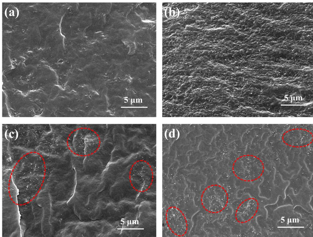
**Figure 3.** SEM images of the G-CNT/EVA composites with (a) 0.3 wt % and (b) 2.0 wt % CNT, respectively. SEM images of the CNT/EVA composites with (c) 0.3 wt % and (d) 2.0 wt % CNT, respectively. The red circles in (c) and (d) refer to the CNT agglomerations.
