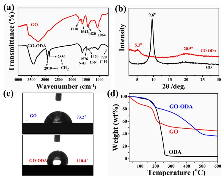
**Figure 2.** (a) Fourier-transform infrared spectroscopy (FTIR) spectra of graphene oxide (GO) and octadecylamine-grafted GO (GO-ODA); (b) X-ray diffraction (XRD) patterns of GO and GO-ODA; (c) Surface water contact angle of GO and GO-ODA; (d) TGA curves of ODA, GO and GO-ODA.
