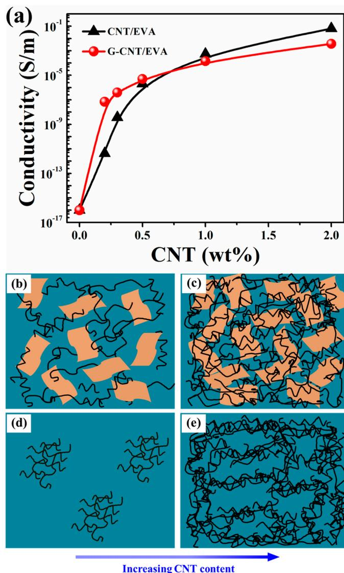
**Figure 5.** (a) Electrical conductivities of the G-CNT/EVA and the CNT/EVA composites. (b) and (c) The scheme of the conductive networks in the G-CNT/EVA composites at low and high CNT contents, respectively. (d) and (e) The scheme of the conductive networks in the CNT/EVA composites at low and high CNT contents, respectively.
