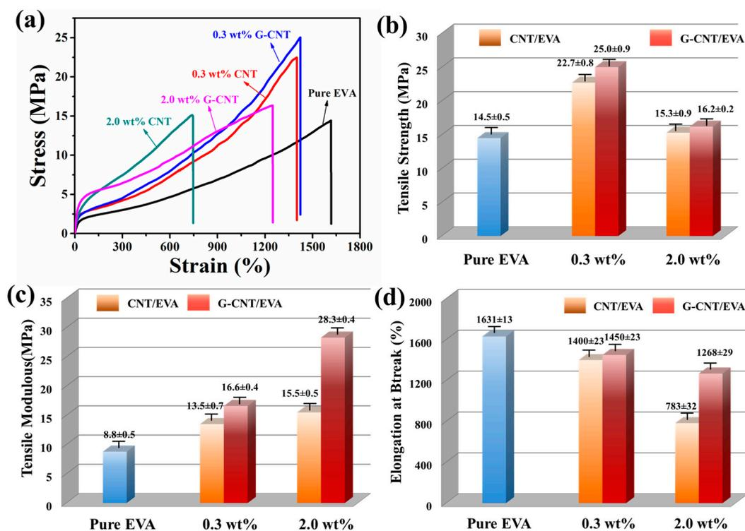
**Figure 4.** (a) Typical stress–strain curves of pure ethylene vinyl acetate (EVA) and its composites with various CNT loadings; (b) Tensile strength, (c) Young’s modulus, and (d) elongation at break of pure EVA and its composites.
