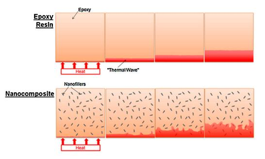
**Figure 3.** Thermal conductivity by graphene in a graphene-polymer composite [29]. Copyright (2016), with permission from Elsevier.
