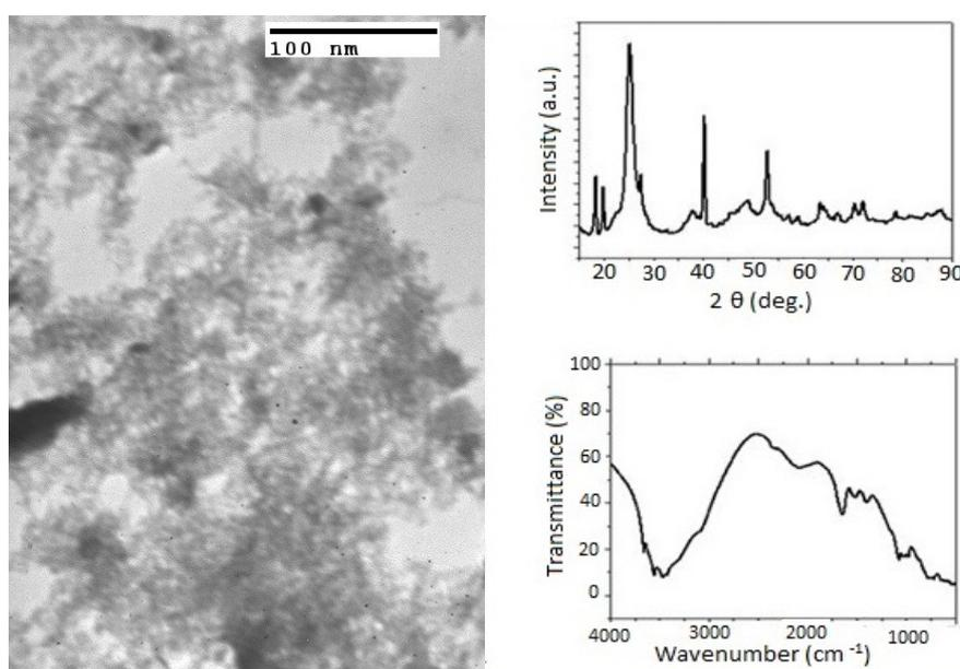
**Figure 1.** XRD, FTIR, and TEM for the prepared Al<sub>2</sub>O<sub>3</sub> nanoparticles.
