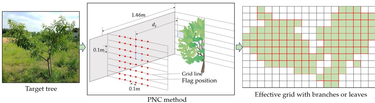
**Figure 2.** Principle of artificial canopy volume measurement.
