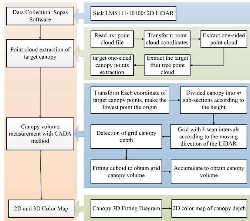
**Figure 4.** LiDAR point cloud processing flow.
