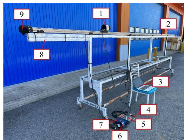
**Figure 1.** Schematic diagram of the fruit tree canopy point cloud data acquisition system: 1. LiDAR; 2. guide rail; 3. computer; 4. LiDAR power supply; 5. stepper motor power supply; 6. stepper motor controller; 7. stepper motor driver; 8. mobile platform; 9. stepper motor.
