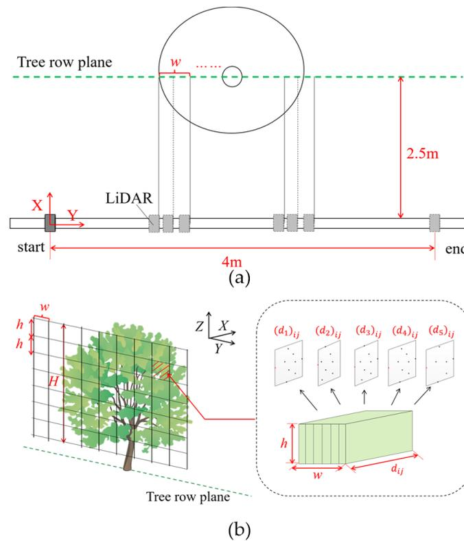
**Figure 3.** Detection principle of the CADA method: (a) Lidar data acquisition; (b) canopy volume calculation.
