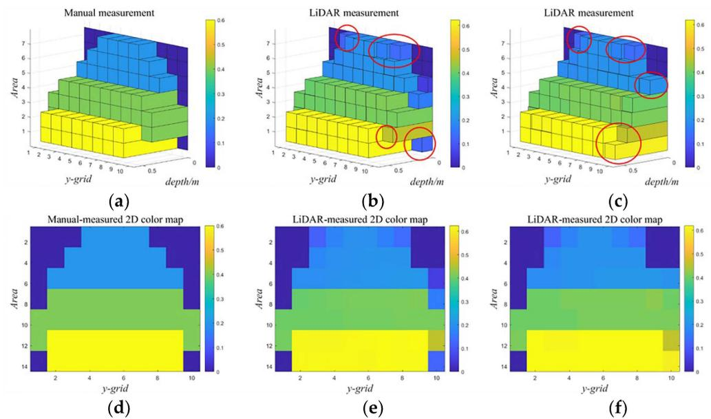
**Figure 7.** LiDAR measurement vs. ground truth: (a) manually measured 3D colour map; (b) LiDAR-measured 3D colour map (average depth); (c) LiDAR-measured 3D colour map (maximum depth); (d) manually measured 2D colour map; (e) LiDAR-measured 2D colour map (average depth); (f) LiDAR-measured 2D colour map (maximum depth). Note: The red circles in the figure refer to the edge grids that can detect the canopy depth.
