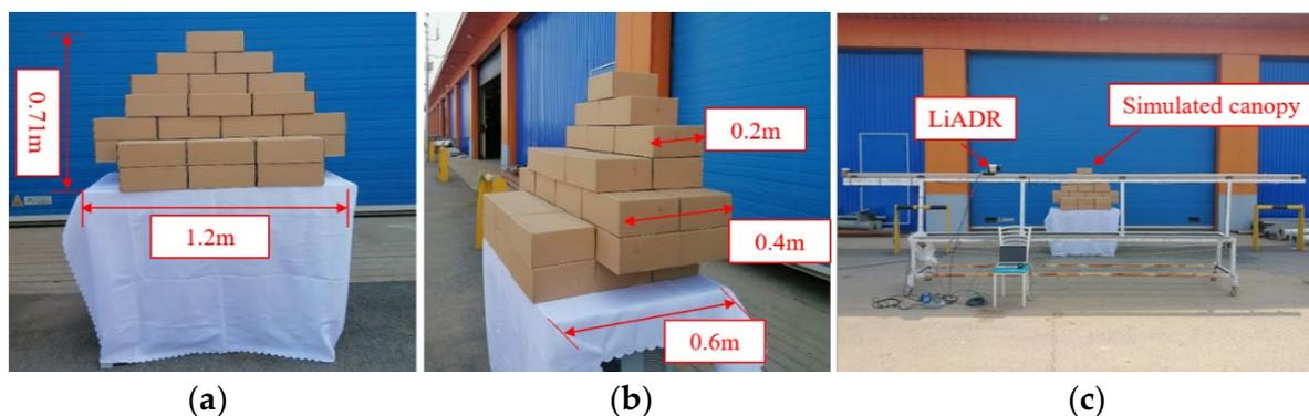
**Figure 5.** Simulated canopy test: (a) canopy front; (b) canopy side; (c) LiDAR detection process.
