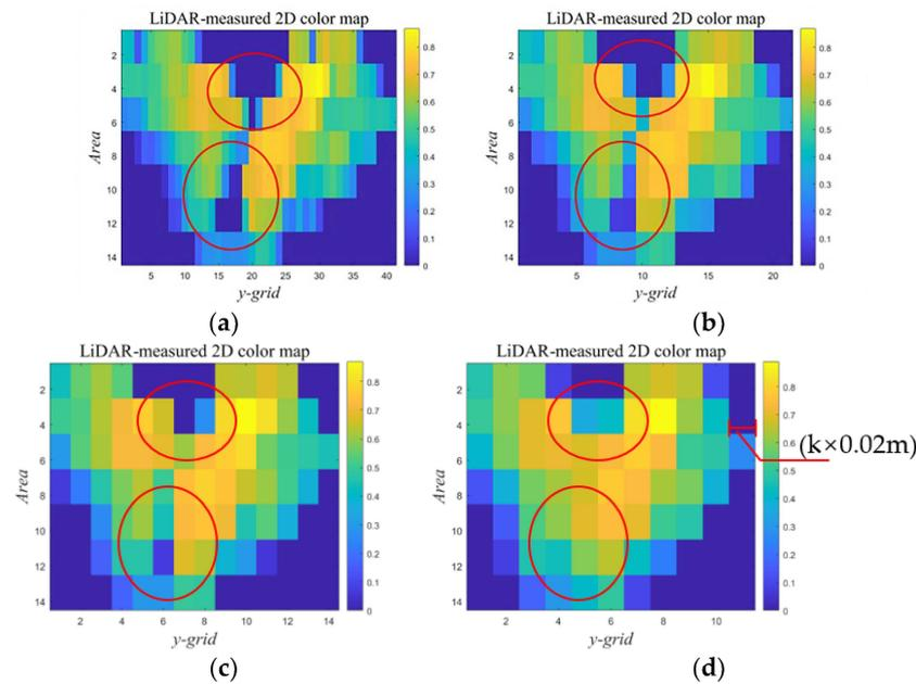
**Figure 9.** 2D depth colour map of canopy LiDAR detection under different mesh widths: (a)  $k = 2$ ; (b)  $k = 4$ ; (c)  $k = 6$ ; (d)  $k = 8$ . Note: The red circles in the figure refer to the grid with the depth of 0 inside the canopy.
