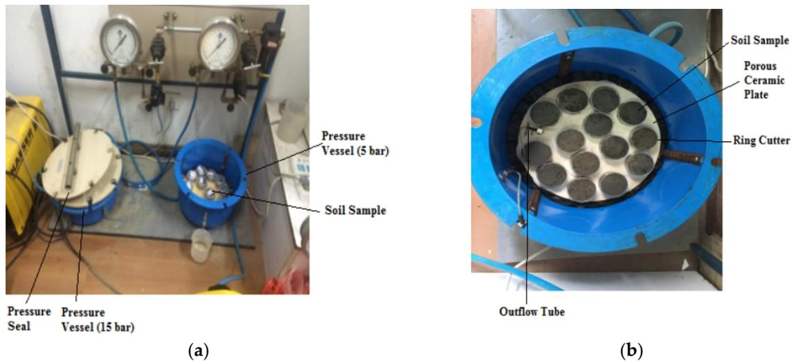
**Figure 1.** (a) Pressure plate testing using the Pressure Vessel 1500; (b) soil specimens on a 1 bar ceramic plate.
