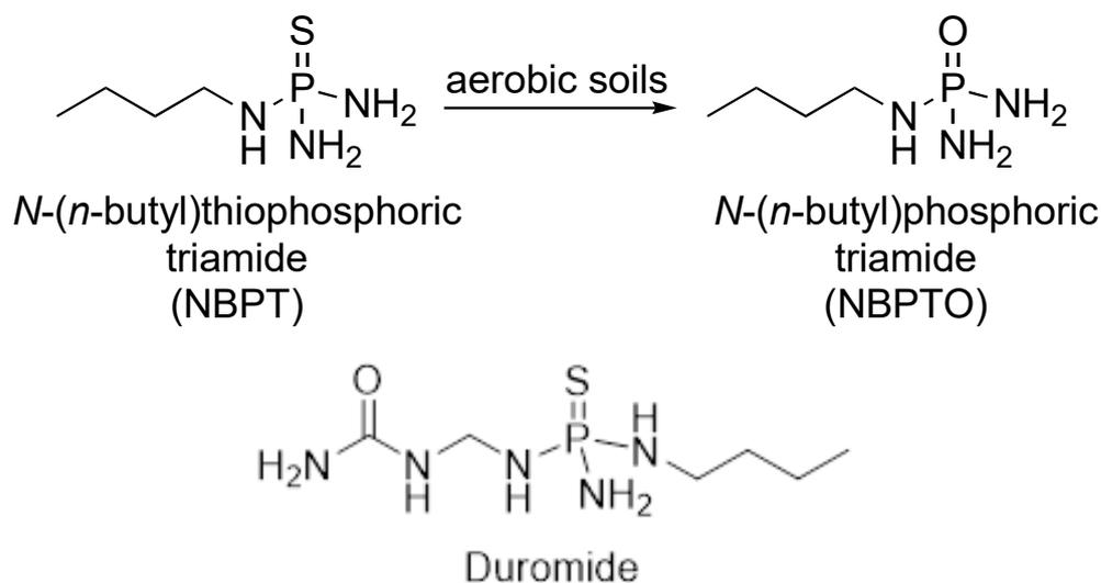
**Figure 3.** Hydrolysis of *N*-(*n*-butyl) thiophosphoric triamide (NBPT) to *N*-(*n*-butyl) phosphoric triamide (NBPTO) in soils (left). Structure of Duromide (ANVOL, Koch) (right).
