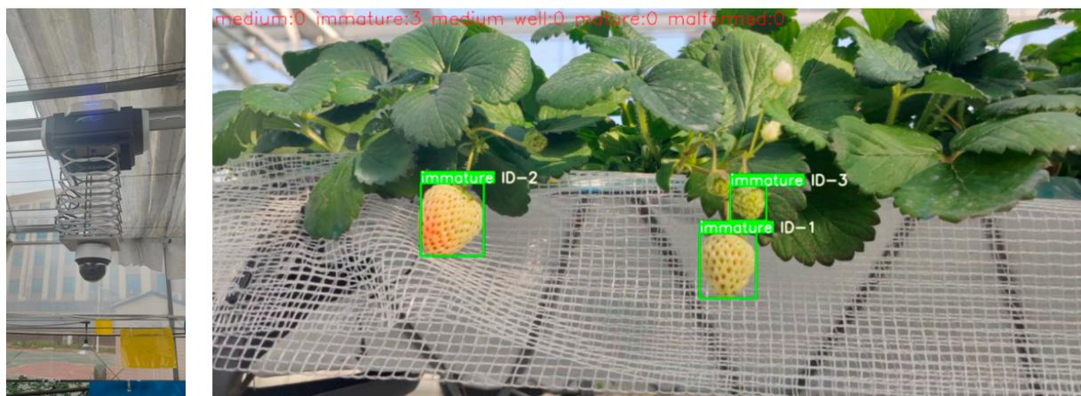
**Figure 16.** Identification and assessment of strawberry maturity via inspection robot.
