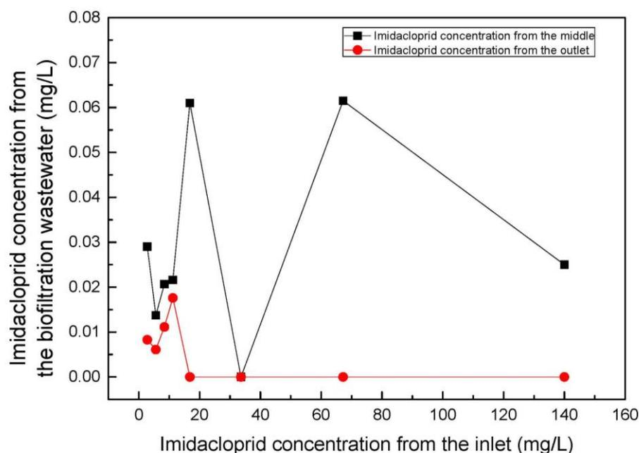
**Figure 3.** Variation in pesticide residues in wastewater from the biofilter system.
